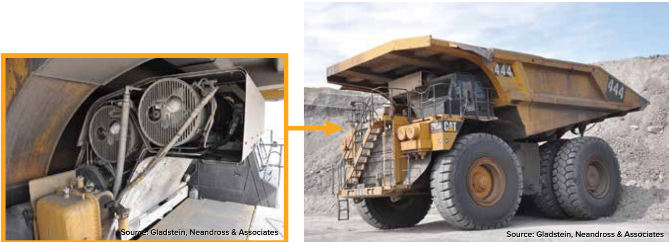
Figure 23. Close-up of LNG fuel tanks in CAT 793 dual-fuel haul truck at Belle Ayr Mine
